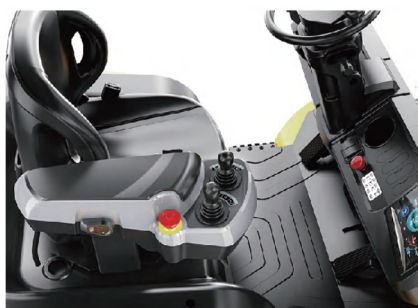
Shock-absorbing seats to eliminate fatigue, equipped with OPS switch and seat occupancy sensor
